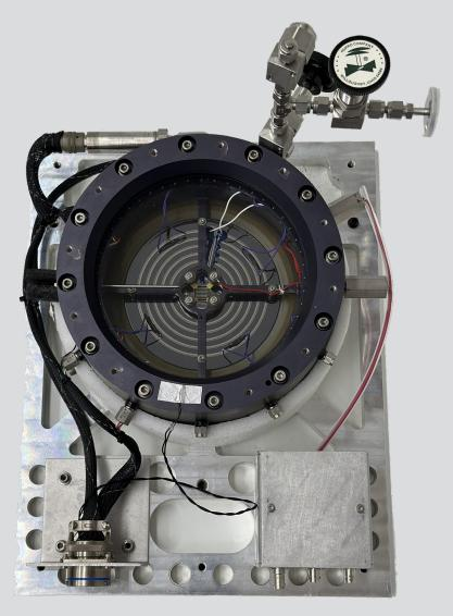
Multi-Scale Heat Transfer Laboratory at WPI test chamber for EHD conduction driven liquid film flow boiling in the presence of dielectrophoretic force, flown in micro-gravity flights
